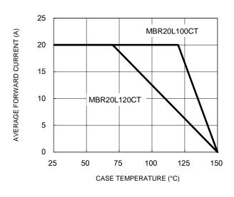
Fig.1 Forward Current Derating Curve
